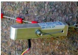
The Circumference Dendrometer 1 is the simple version for the measurement of circumference changes of plants. The sensor is mounted by means of a stem embracing cable wire. The cable wire consists of a special material (purpose specific alloy), with the lowest thermal expansion coefficient available. Slide rings reduce the friction and pressure between the wire cable and the tree bark.
