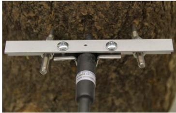
The DRW is the ruggedized version of the DR1 dendrometer type. In addition to the features of the simple DR1 version, the DRW dendrometer is modified for the use under especially harsh environmental conditions. A soft, weather-resistant rubber coating, protects the whole sensor from ingress of water and solid particles.
