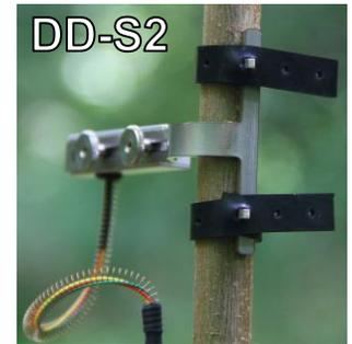
The DD-S Type dendrometers are designed specifically for agricultural plants, small trees and branches (diameter < 5 cm). Due to the optimized mounting method, the dendrometer provides stable readings also for very small plants. The sensor remains stable fixed at the measuring point without exerting excessive pressure on the measuring point. The sensor is available in two versions: DD-S1 with standard mounting frame, DD-S2 with quick mount frame
