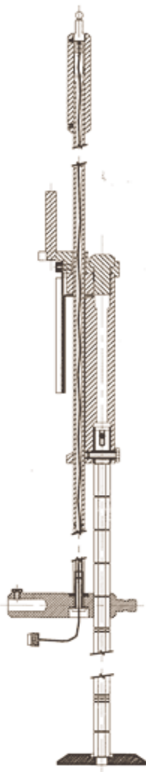
Figure 1: TSR Schematic With Bucket Meter Adaptor Attached
