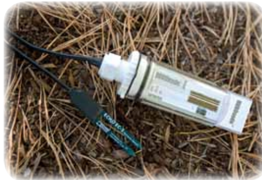
HOBOnode sensors, such as the Soil Moisture Sensor shown above, provide research-grade performance. Their compact design makes for easy installation in the field.
