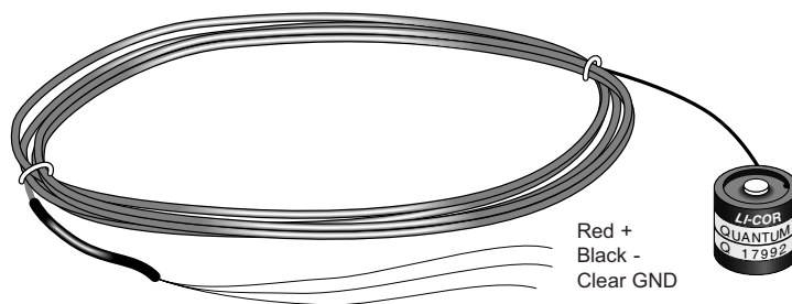
LI190SB Quantum Sensor. The LI200X has a similar appearance and identical wiring.
