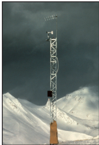
Meteorological conditions measured at Lake Louise, Alberta, Canada are telemetered via phone-to-RF link to a base station.
