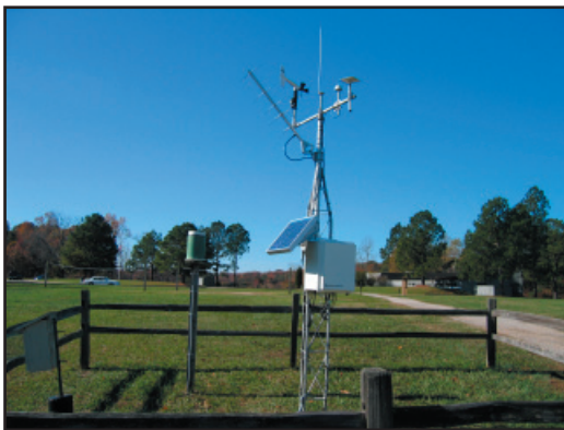
This station for the National Estuarine Research Reserve (NERR) in Virginia transmits data via our GOES satellite transmitter.
