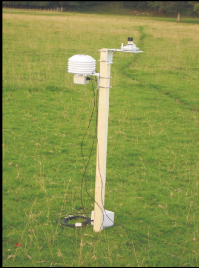
Fig. 1. Skye DataHog set up in field with light sensor and temperature/ relative humidity sensor
