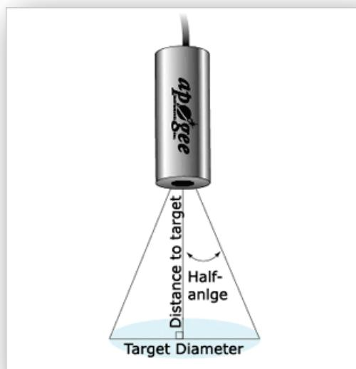
Sensor FOV, distance to target, and sensor mounting angle in relation to the target will determine target area. Different mounting geometries (distance and angle combinations) produce different target shapes and areas, as shown below.
