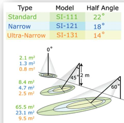
A simple FOV calculator for determining target dimensions based on infrared radiometer model, mounting height, and mounting angle, is available on the Apogee website: <http://www.apogeeinstruments.com/using-your-apogee-instruments-infrared-radiometer/>.
