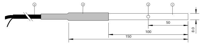
Figure 1 ST01 Soil Temperature Sensor: The sensor consists of a stainless steel needle (1) with a temperature sensor (2) (normally Pt100, also Pt500 and Pt1000 available). The Pt elements are connected in a 4-wire configuration. The Teflon cabling (3) is welded (4) to the stainless steel. All dimensions are in mm.
