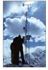
Data measured by this weather station near Aspen, Colorado is used in avalanche forecasting.
