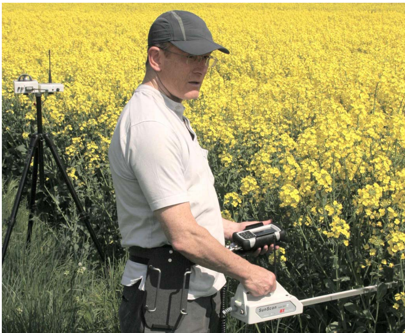
SunScan Probe (radio version) and PDA, with radio-linked BF3 Sunshine Sensor mounted on tripod
