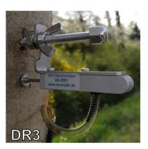
DR-Type dendrometers are fixed with one (DR3) or two special screws (DR1 and DR2), anchored in the trunk wood. The changes outside of the trunk wood correspond to radial growth and water status related, diurnal diameter variation. The arrangement ensures high stability for long-term measurements.
