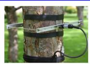
The DDW is the ruggedized version of the DD-L1 dendrometer type. In addition to the features of the DD-L1 version, the DDW dendrometer is modified for the use under especially harsh environmental conditions. A soft, weather-resistant rubber coating, protects the whole sensor from ingress of water and solid particles.
