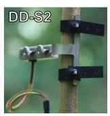
The DD-S Type dendrometers are designed specifically for agricultural plants, small trees and branches (diameter < 5 cm). Due to the optimized mounting method, the dendrometer provides stable readings also for very small plants. The sensor remains stable fixed at the measuring point without exerting excessive pressure on the measuring point. The sensor is available in two versions: DD-S1 with standard mounting frame, DD-S2 with quick mount frame
