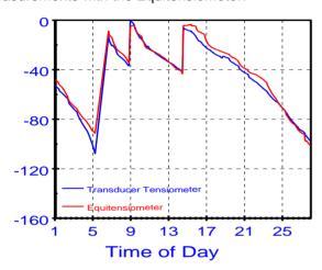
Fig. 2: Comparing the sensitivity of the EQ15 (red line) with transducer tensiometer (blue line). The soil was periodically irrigated. Either during the wetting or drying phases there were no significant differences between both sensors.
