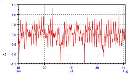
Fig. 1 Vertical temperature gradients of a 40-year old spruce tree, measured with a Granier sensor with the heating turned off.
