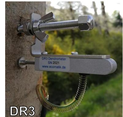
DR-Type dendrometers are fixed with one (DR3) or two special screws (DR1 and DR2), anchored in the trunk wood. The changes outside of the trunk wood correspond to radial growth and water status related, diurnal diameter variation. The arrangement ensures high stability for long-term measurements.
