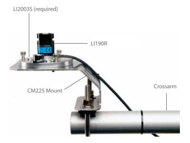
The CM225 attaches to a crossarm by placing the U-bolt in the holes on the bottom of the bracket.
