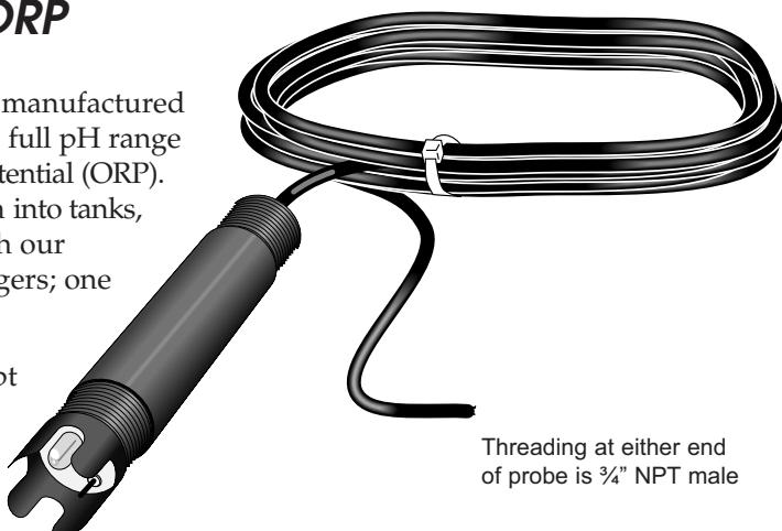
The sensors feature a plunger-style\* pH glass electrode allowing them to be mounted at any angle. The porous Teflon® liquid junction\*\* is less susceptible to clogging as compared to conventional reference junctions. A titanium ground rod runs inside the PPS outer body to eliminate ground loop errors. An internal amplifier boosts the signal, decreasing signal interference.
