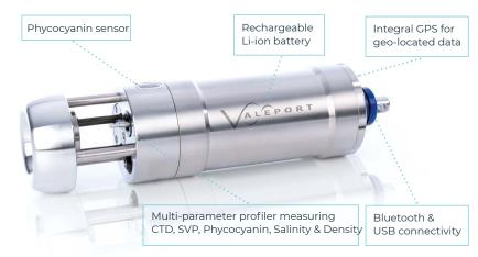
Valeport's Hyperion Fluorometer sensor range, when combined with SWiFT, delivers high performance measurements of Phycocyanin in a compact & robust package.
